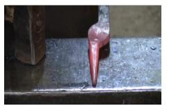
1. Draw out and taper the jaw end on each blank.
