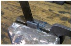
1. Heat the ends of the Quick Bolt Tong blanks. Clamp in a vise and split using a sharp hot chisel
