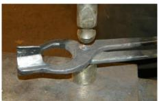
4. Drill a 5/16" diameter hole and rivet both blanks together using the rivet included in your order. You have finished!
