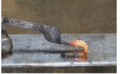
**4.** Shape the jaw on the edge of the anvil to thin and curl the end.
