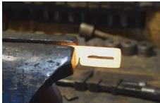
2. Heat the jaw end and clamp in vise with the groove facing down and lined up with the edge of the vise.
