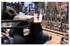
7. Reheat, put in vise, and use a wrench/tongs to twist the jaw counterclockwise 90 degrees. Use a hammer to straighten as necessary.
