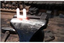
5. Heat up Part "B" and place it in the vise with the rein facing left and the bottom of the "U" about 1/4" from the top of the vise. 6. Bend backwards with hammer.
