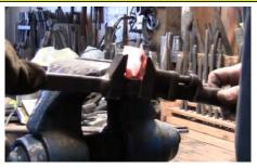
**3.** Reheat and twist the jaw 90 degrees counter clockwise
