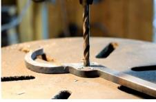
**3.** Drill a hole to fit your rivet.
