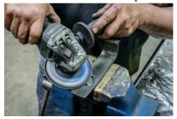
5. Remove any burrs from each of the drilled holes.
