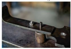
7. Complete the rivet, remove the bolt, and rivet the second hole.
