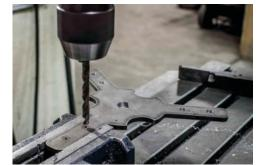
3. Drill a total of six 5/16" holes in the arms of the base plate.
