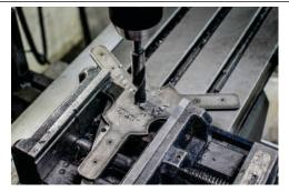
2. Drill a 5/8" hole in the center hole of the base plate.
