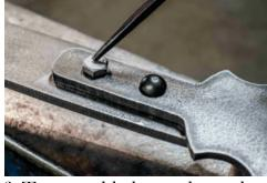
6. To assemble legs to base plate, align the holes from each. Fasten bolt into one set of holes Insert the rivet into remaining hole.
