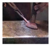
5. Use a fuller tool to make grooves for leaf veins
