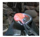
7. Use a leafing hammer and cupping tool to shape the edges of the leaves
