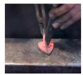
**3.** Use a fuller tool to make a groove down the center of
