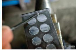
3. Flip everything over and insert each of the tabs into the remaining Side Support. Be sure that the bottom is on the correct side and check that there is no gap. Lightly peen the tabs over. Once everything is in place, use harder blows to finish peening out the tabs on both sides.
