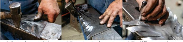
1. Shape and texture each piece prior to assembly. Use various hammers and texturing tools to add dimension to your tree.
