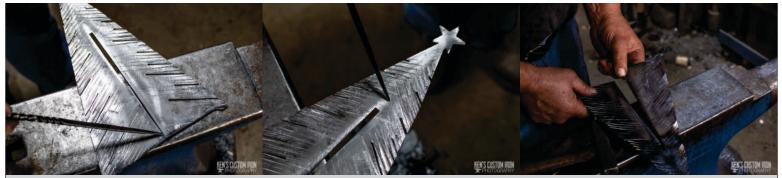
Any hammering you do to the tree cause stretching, which will close up the slots.
