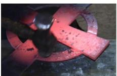
**2.** Texture the ring with a ball-pein hammer using rapid, light blows.
