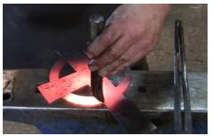
**1.** On the back piece, use a butcher tool to fuller in a groove where the ring meets the cross.
