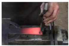
**3.** Use a hot set or an edging chisel and fuller in a groove at the end of each arm of the cross.
