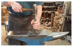
**1.** Use a hammer and chisel to separate the petals.
