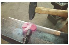
**2.** Heat the flower blank and texture it with a cross-peen or ball-peen hammer.
