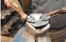
**2.** Shape the petals in a cupping tool or swage block.
