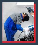
Welding requires an allocated area where PPE includes a facemask with UV protection for the eyes and skin coverage that protects from burns both from heat or UV as well as sparks or splatter.
