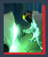
UV Curing (stationery & mobile handheld systems) requires allocated area where PPE includes a face mask with UV protection for the eyes and skin coverage for UV protection.
