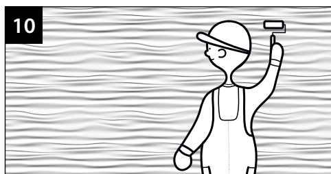
10 Before painting, panels should be prime by WeldPrimer by using a velor roller.
