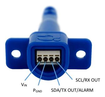
Note: For  $I^2C$  communication, external pull-up resistors to +3.3V for SDA and SCL are required. The F200 does not have internal pull-up resistors.
