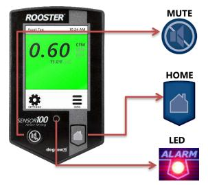
Returns the user to the home screen when pushed from any menu or info screen. \* Cannot be used to abort ome critical system functions.\*
