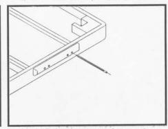
While holding the 'Wood Conversion Plate' in place, use a pencil or pen to mark the location of the large holes in the 'Wood Conversion Plate' on the end of the Massage Table.
