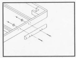
Using the large washers and 3/16" hex nut, secure the 'Wood Conversion Plate' to the end of the table. Before tightening make sure plate is positioned parallel to the bottom edge of the massage table.
