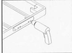
With the drill & 3/8" drill bit, drill holes completely through the end of the massage table using the outer holes in the 'Wood Conversion Plate' as a guide. Be sure to hold the drill as level and straight as possible so the new 'Plug-in Face Space' will adjust properly.
