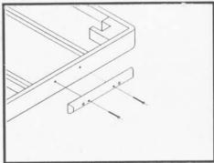
Position the 'Wood Conversion Plate' on the end of the Massage Table by inserting the screws through the existing holes.
