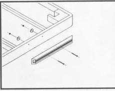
Remove existing mounting plate and screws from the massage table and disgard.
