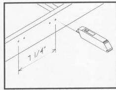
Remove the 'Wood Conversion Plate'. Use a knife to cut a small "X" in the vinyl at the pencil marks you just made on the end of the massage table.
