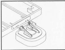
Line up the steel rods from the new 'Plug-in Face Space' with the 3/8" holes that you just drilled to check for a proper fit.
