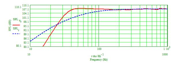
You can see f3 is about 33 Hz, f6 is 30 Hz and f10 is  $\sim$ 27 Hz. The output SPL will be less than the 107 dB after BSC is incorporated. The system is tuned to 32 Hz. This 50-watt input causes the mid-woofers to reach Xmax +15% at 48 Hz with the port's peak air velocity hitting 17 m/s at just over 30 Hz.
