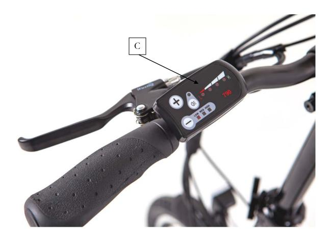
The red lights dots will indicate the battery level (you can check also by pressing the other indicator that is located on the battery). You can use the *Plus* and the *Minus* buttons to change the motor assist level. On low you get less power from the motor and you need to use more the pedals and on high you will get the full power from the electric bike. The light button is to turn on and off the front and the back light.
