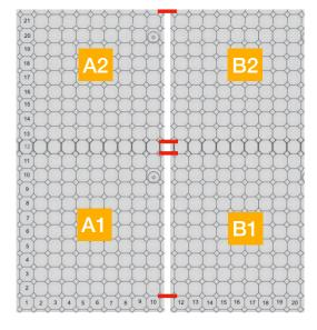
b. Connect A1 to B1, A2 to B2 by inserting the METAL CONNECTOR PIECES along the middle column where the PLASTIC CONNECTOR CLIPS were inserted in step 3a
