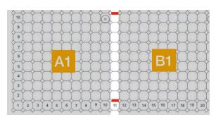
b. Connect A1 to B1, A2 to B2 by inserting the METAL CONNECTOR PIECES along the middle column where the PLASTIC CONNECTOR CLIPS were inserted in step
