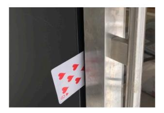
Check the door rubber seal by sliding paper in between seal and housing.
