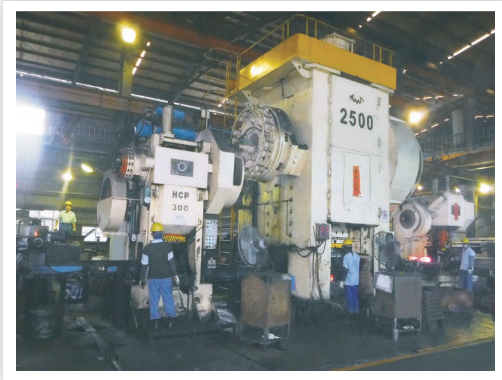
沖床及感應加熱設備鍛造設備操作現場 ▲ HIGH SPEED PNEUMATIC PRESS EQUIPPED WITH INDUCTION HEATER
