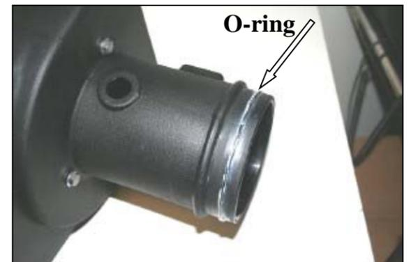
**6.** Install the O-ring (#17) into the groove on the Cool Air Box as shown. Apply a *light* coat of the supplied grease onto the O-ring.
