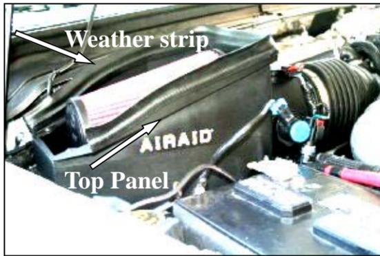
**11.** Install the Airaid Premium Filter (#1) onto the filter adapter, and tighten the hose clamp. Next install the Top Panel (#3) onto the top of the Cool Air Box using six 8-32x3/8" button head bolts (#9), and #8 flat washers (#10). Install the weather strip (#5) onto the edge of the top panel as shown
