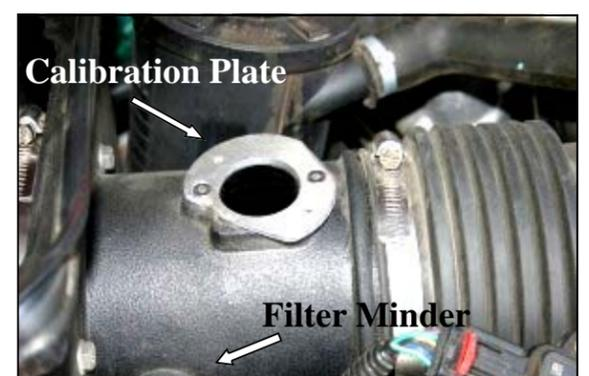
**9. A.)** Install the Calibration Plate onto the Cool Air Box using two 8-32 x 1/2" Flat Head Screws (#14). **B.)** Reinstall the factory grommet, and filter minder into the Cool Air Box, and then reconnect the filter minder wiring harness.
