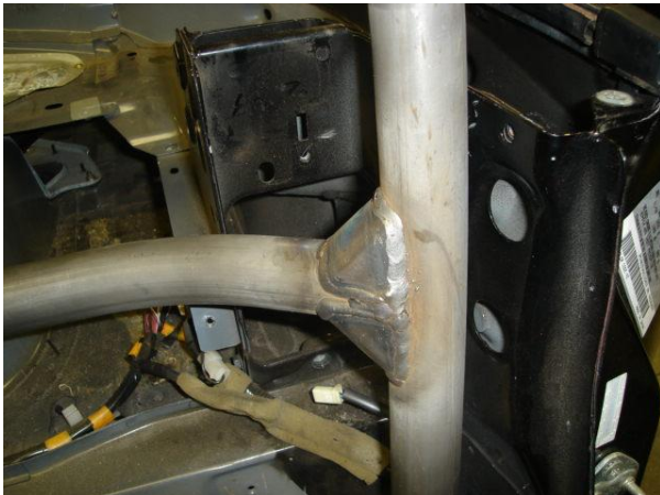
Note the angle of the main hoop
