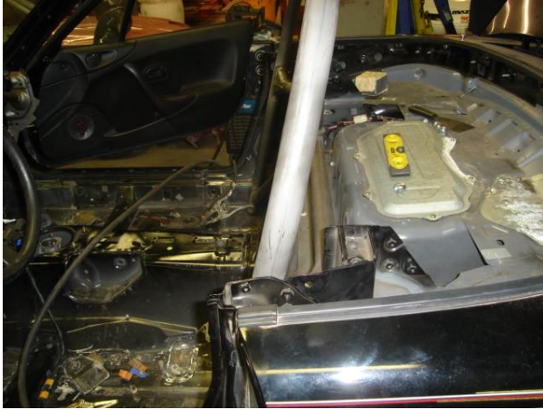
Note the angle of the main hoop
