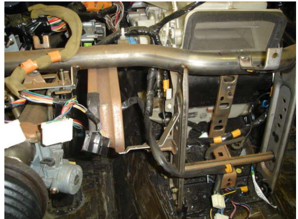
Some braces need to be removed in the center dash area
