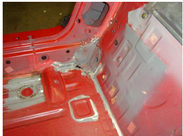
The oem rear gusset has been removed. The "camel hump" remains
