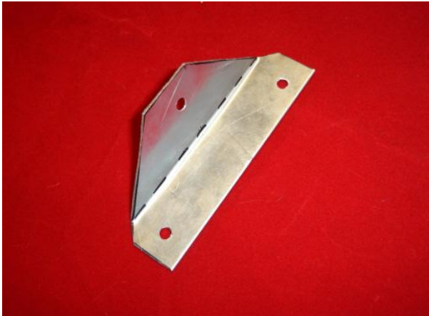
Defroster duct mounting tab
