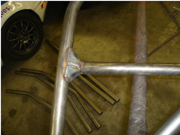
This shows the 3-dimensional gussets installed in the main hoop area
