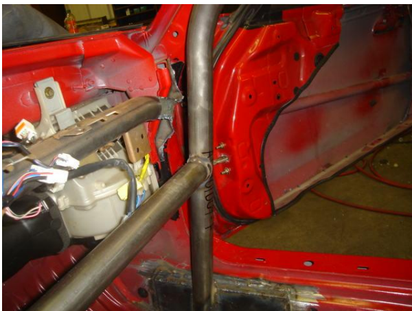
This pic shows a completed front section prior to installing the dash pad and door bars
