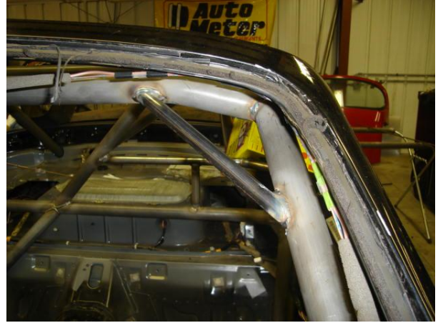
The optional windshield diagonal bar acts as a stiffener and also as a handle for getting out of the car.
