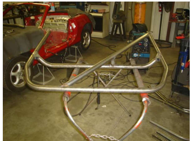
This main hoop is completely welded and ready for installation
