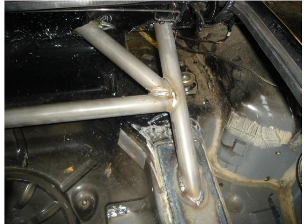
Note how all 3 tubes are welded together in the trunk
