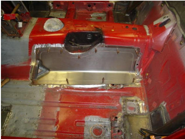
This East Street Racing Floor Notch Out Panel is available from Advanced Autosports. It provides additional floor clearance for larger seats.
