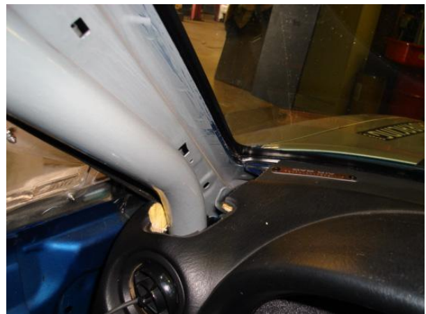
Trim the dash as close to the bars as possible
