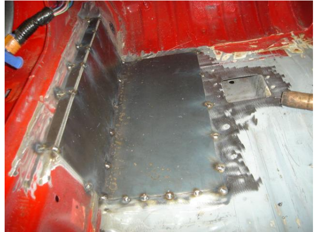
Picture of drivers front footings tack welded in place
