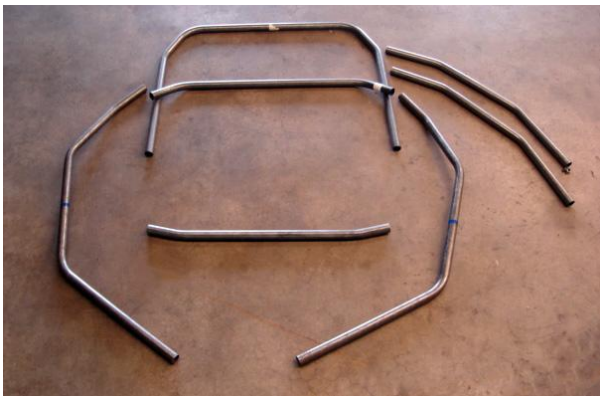
This pic shows the tubing for the Advanced Autosports basic roll cage kit
