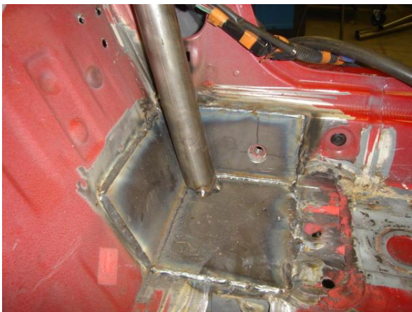
2 pix of the main hoop footing, NOTE: hole in side plate for access to factory seat belt hole
