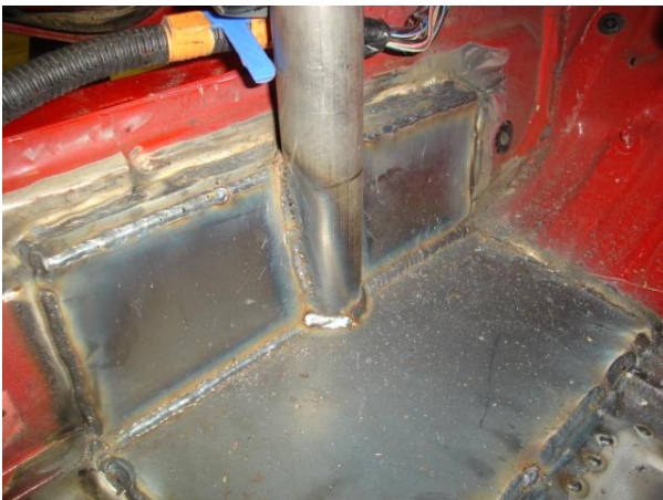
This left front bar leaves plenty of room for the drivers feet and the factory dead pedal.
