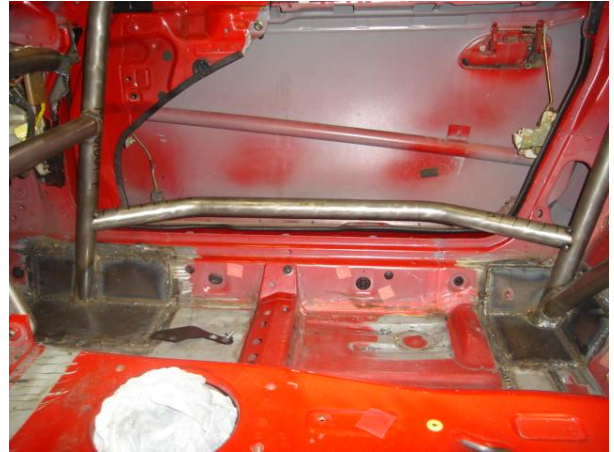
Make sure the door will close before final welding of the lower door bar.
