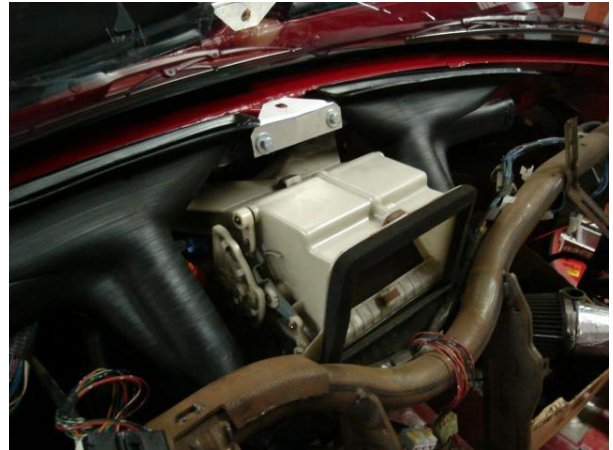
The little silver bracket holds the defroster ducts in the proper position
