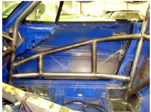
For the most strength, the NASCAR bar should attach to the upright as close to the harness bar as possible.
