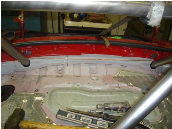
The curvature of the body will fool the eye into misaligning the 3 holes in the rear bulkhead. This straight rod helps with proper alignment.
