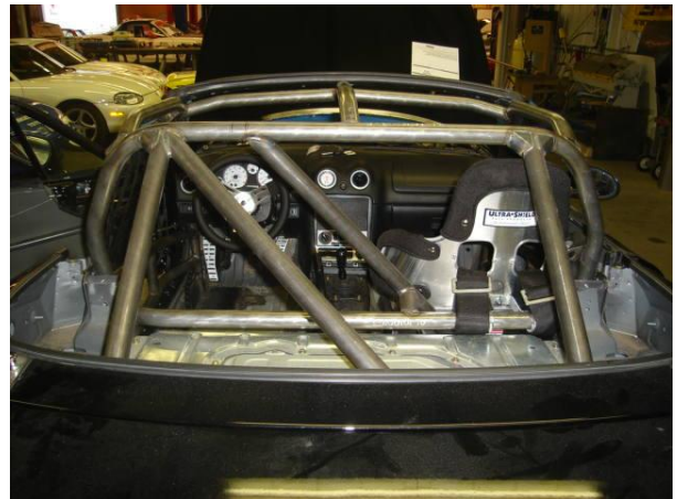
You may wish to offset the roof bar slightly for additional helmet clearance.
