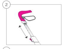
Press on the height adjustment button on the frame with one hand while pulling the handle with the other
