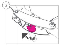
3. If you are in doubt whether the folding mechanism is correctly locked e.g. in a noisy environment, please check that the locking hook under the seat is properly locked into place.
