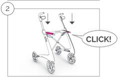
Push downwards on the outer rails of the seat in one swift motion, until you hear a significant click from the locking mechanism.
