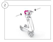
2. To ensure that the rollator is completely folded, push the handles toward each other.
