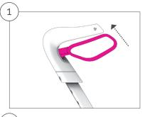
Pull the brake levers upwards to activate the brake. The lever moves back to the neutral position when the
