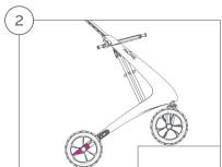
Even though Carbon Ultralight is the world's lightest walker and therefore is easier to lift, it is equipped with a kerb lifter that makes it easier to get over smaller obstacles like kerbs and low steps. This is particularly helpful if heavy objects are transported in a front-mounted basket or bag.
