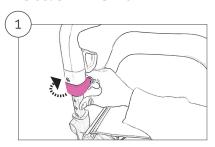
1-2. Grab the mounting clip and turn it clockwise until it releases from the handle bar. Repeat the same steps on the right side, but turn the mounting clip counter-clockwise until it releases from the handle bar.
