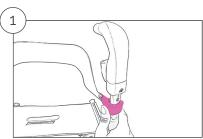
Repeat step 1 and 2 and push instead the mounting clip clockwise until you hear a 'click' and the clip is fastened.
