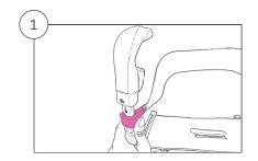
1. Attach the mounting clip on the backrest to the handle bar on the rollator. Hold the clip as shown on the illustration. Push the clip towards the handle bar until it is attached around the bar. Be aware that the clips can still slide up and down the bar at this point.
