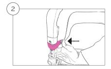
2. Find the preferred height and turn the clip counter clockwise until you hear a 'click'. Be aware that the small peak on the inside of the clips has to fit into one of the holes on the handle bar.
