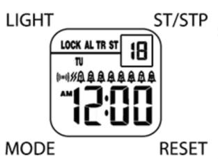
To change the time from 24 Hour Format to AM/PM Format, Press ST/STP when in the Time Mode.
