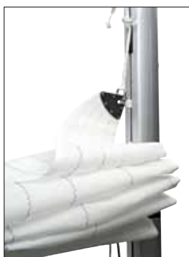
2) The sliders will pass the sail entry all the way down to the tack.
