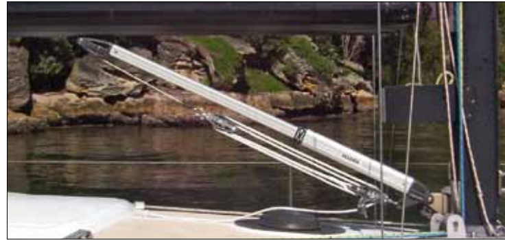
Rodkicker 05 operated at the mast.
