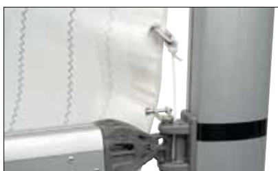
1) Tie the pre-feeder to the boom bracket.
