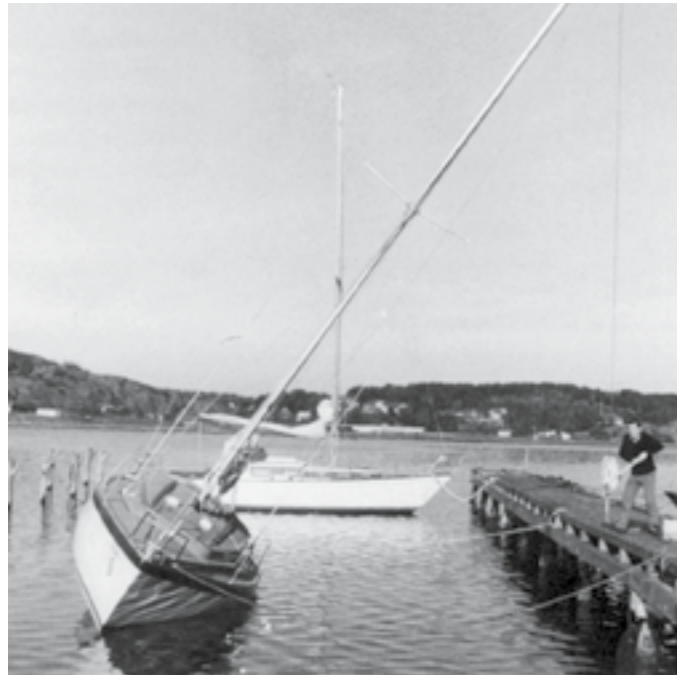
Heeling test in 1965. The righting moment of the boat is measured by 30° heel.
