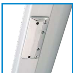
The forestay load is absorbed by a stainless support underneath the cross beam.
