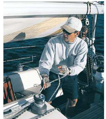
If necessary, apply more main halyard tension.
