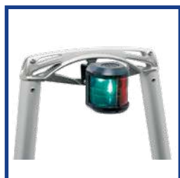
The bridge wire is secured in a slot on top of the bridge support. All prepared for navigational lights.
