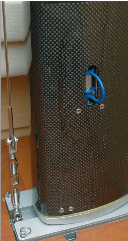
The hose is stored in a hose garage...
