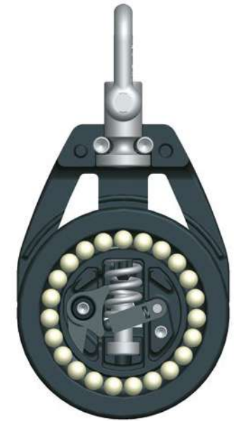
Automatic ratchet block, high load. When the load on the block increases the ratchet engages and the sheave is locked in one direction.
