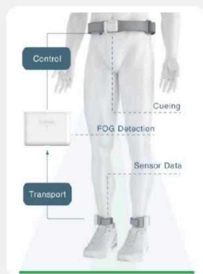
Real-time monitoring of gait through wearable sensors
