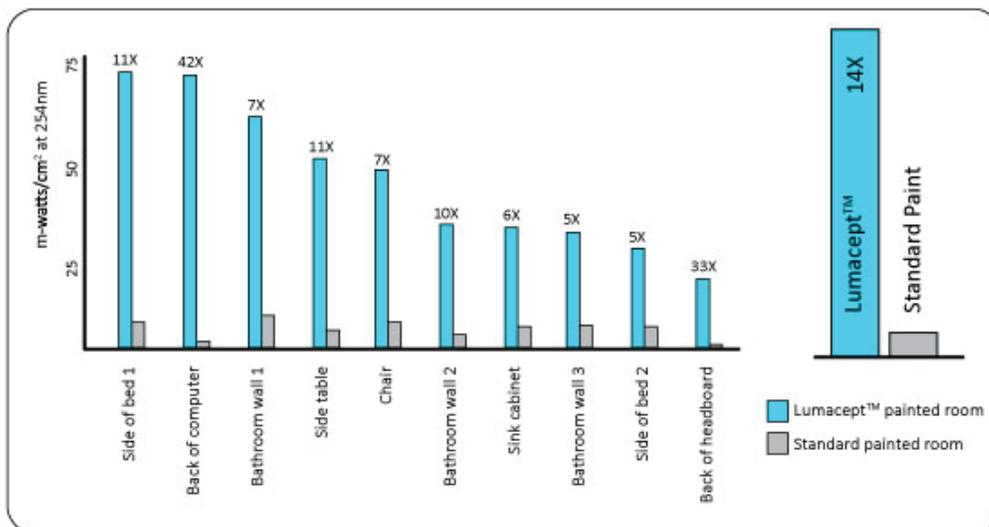
Figure 2. Measurements of UV intensity were taken on various indirect surfaces throughout a hospital room, both with and without the use of Lumacept UV-reflective coatings.
