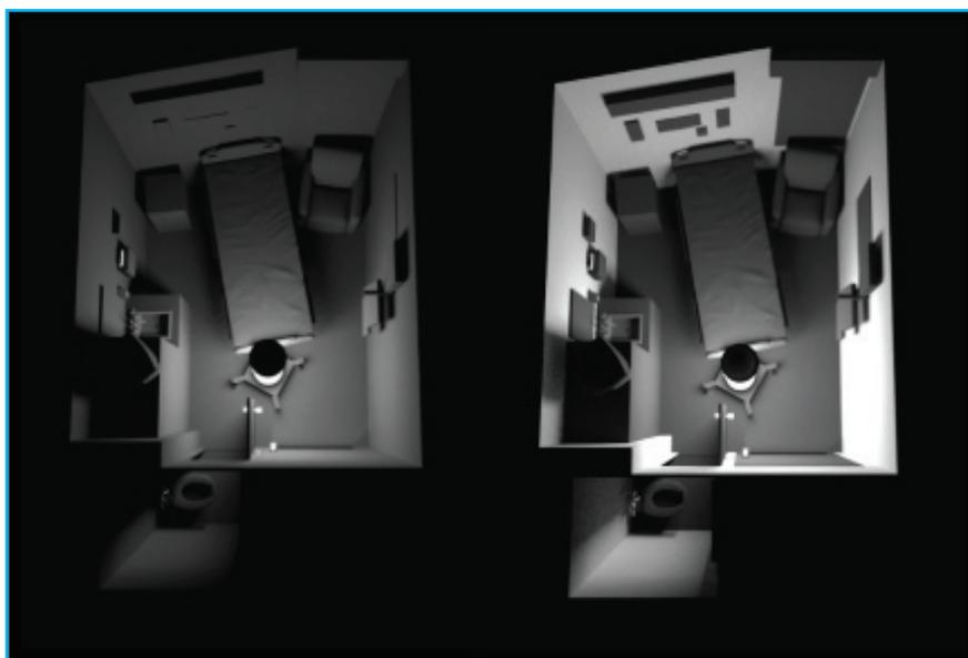
Figure 5. Images from a LumaSim 3D model showing the relative level of UV intensity in a typical hospital room. The room on the left has standard wall paint while the room on the right has UV-reflective paint.
