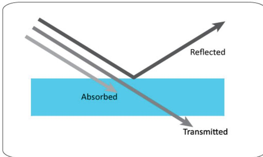
Figure 1. UV light is absorbed, transmitted, or reflected by surfaces.
