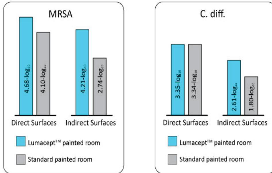
Figure 4. Results from a study of Lumacept UV-reflective coatings using a fixed-cycle device. These results show a significant improvement in log-reduction, especially for those areas not directly illuminated by the device.
