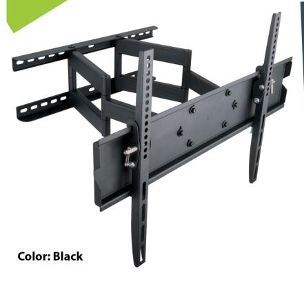
The full-motion wall mount with vesa hole up to 800x400 for most 37"-70" tv up to 60kg.this mount extends out 500mm from wall and places only 115mm to wall when retracted. It can swivel up to 90 degree left or right and 0~-12 degree tilt for up and down meantime it can provide 3 degree horizontal adjustment to ensure it is perfectly level.
