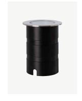
Category Landscaping Light Colour / Finish Satin nickel Materials Aluminium Power Rating 13W Voltage 24V 1180 lumens Light Output 3000K Colour Temp. DIA98 x D120 Dimensions (mm) DIA**81** x H**96** Cutout (mm)
