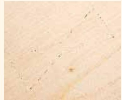
An inlaid patch with matching grain solves the problem and is almost undetectable.
