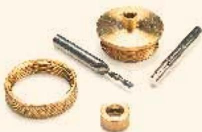
One of the easiest and most reliable ways to fix a defect in the surface of a workpiece is with an inlaid patch. All you need to do is rout away the affected area and replace it with a patch that matches the surrounding grain. Traditionally, these inlays were painstakingly crafted to fit into hand-carved and chiseled recesses. But today, all you need is a plunge router and a simple inlay kit. These tools make it easy to inlay a perfect patch.
