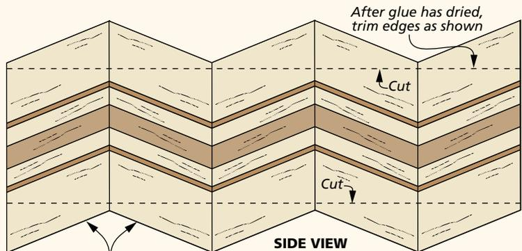
**SECOND:** Alternate orientation and glue back together
