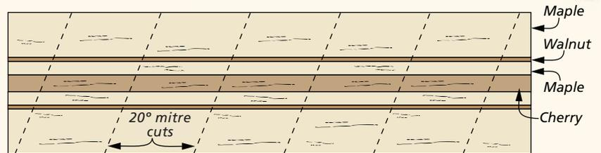
**FIRST:** Sandwich and glue contrasting wood layers together, then make mitred cuts as shown **SIDE VIEW**
