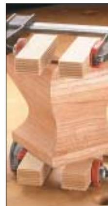
These clamping blocks are plywood so they'll split easily along the plies. And they're glued in place with hide glue, which can be loosened with a little hot water.
