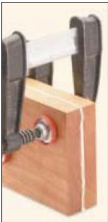
Bracket feet look like they were cut from thick blocks of wood, but these blanks were made with two pieces of 19mm-thick stock.
