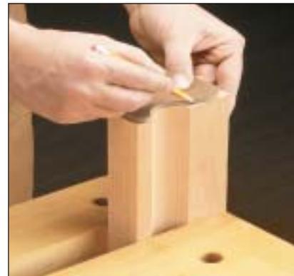
{ Hardboard makes a good, reusable template for the bracket feet profiles, see pattern at left. To position the template on the blank, just line it up with the cove you've already cut.
