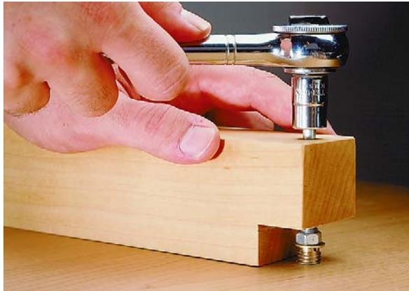
▲ This simple tool makes it easy to install a threaded insert straight. A nylon bushing and a spring help hold the threaded insert upright as it's driven into the workpiece.
