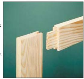
When making a haunched mortise and tenon joint, there's nothing unusual about creating the grooves or the mortises (Steps 1 & 2). Just make sure that the mortises are sized to match the width of the grooves. The tenons are pretty much the same as a traditional tenon too (Steps 3-6). The only difference is the extra shoulder (haunch) on the outside edge.
