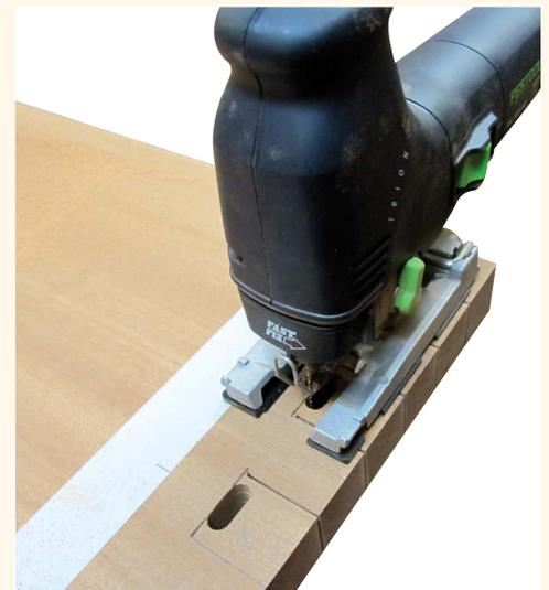
▶ *Square shoulders are cut to create the sides of the pins before the backs are squared off.*
