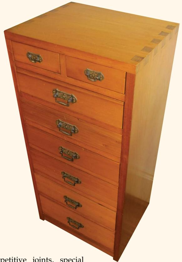
repetitive joints, special attention needs to be paid to which side of the line you are cutting on; it is always the slotted side of the line.
