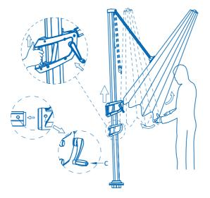
To open the canopy, wind the crank handle (c) in a clockwise direction. To close the canopy, wind the crank handle in an anti clockwise direction.
