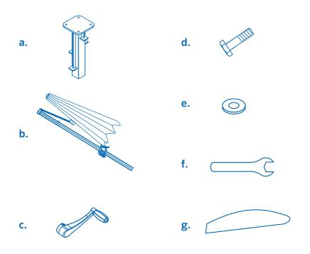
\*This umbrella is designed to be fixed onto the supplied inground mount (a). The inground mount is a steel fixture that must be properly concreted into position. Do not attempt to attach the umbrella until the concrete has fully cured, according to the manufacturer's instructions.
