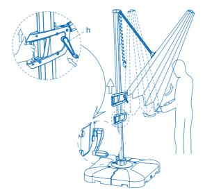
To open the canopy, wind the crank handle (h) in a clockwise direction. To close the canopy, wind the crank handle in an anti clockwise direction.
