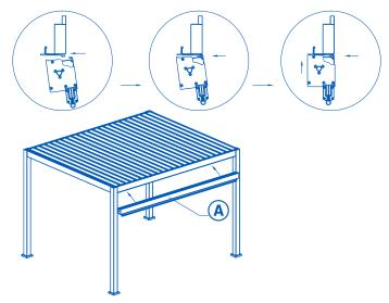
Affix the four **hex screws (F)** into the Blind housing Assembly (A) tightly with **allen key (G)**. Ensure all four screws are spaced evenly apart.
