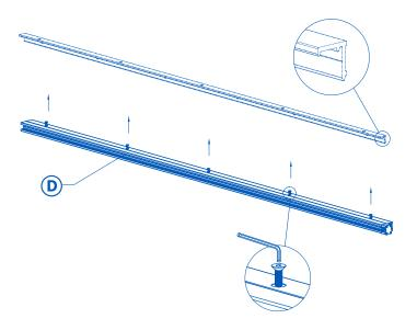
In order to install the rectangular aluminium profile on the vertical post correctly, you can make the use of the positioning rib on the top profile as illustrated. Insert 6 x Tek screws (E) into the aluminum channel and into the vertical post.
