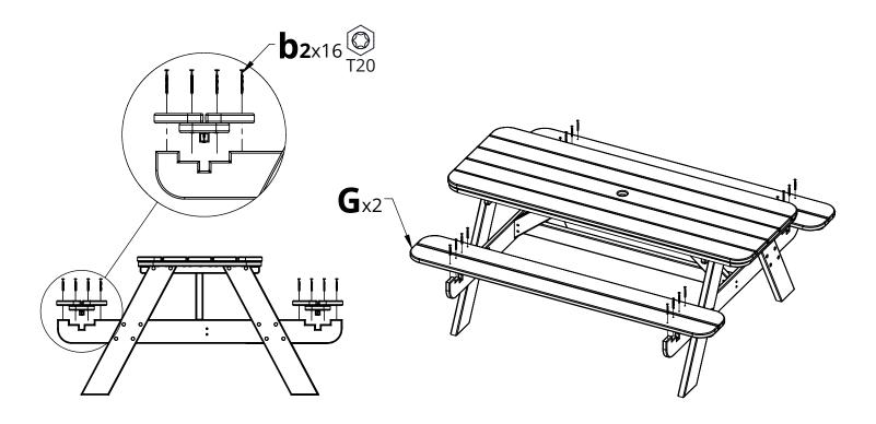
**5.** Rotate the assembly as shown & connect Parts G
