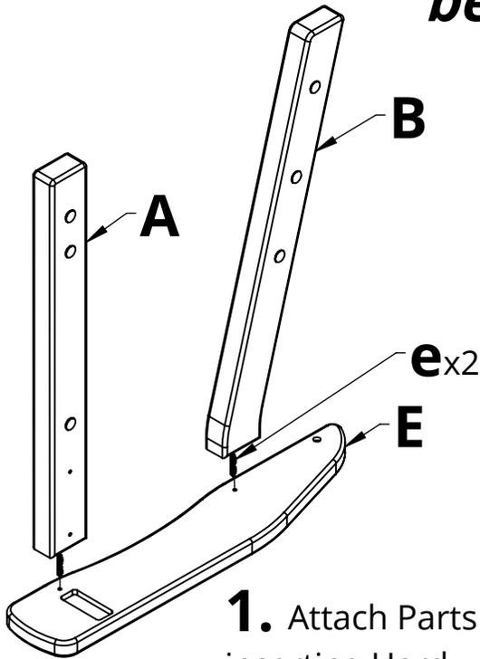
1. Attach Parts A & B to Part E by inserting Hardware e into the pre-drilled holes and rotating Parts A & B clockwise, stopping when the assembly is tight
