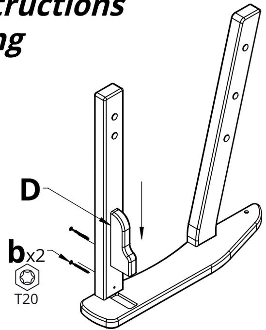
2. Attach Part D to the previous assemblies using Hardware b
