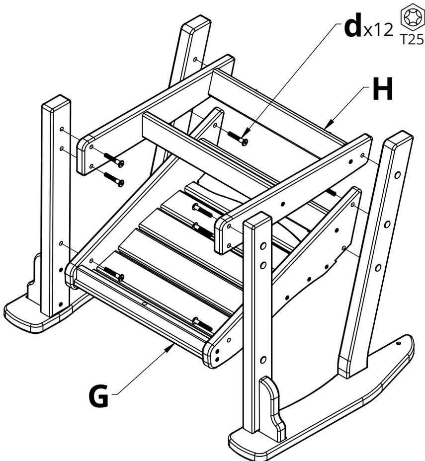
4. Attach Parts H & I to the previous assemblies using Hardware d, this step is made easier if performed with the assembly upside down
