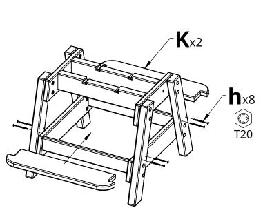
**3.** Attach Part K to the previous assembly using Hardware h
