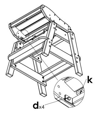
**5.** Attach Part D to Hardware k using Hardware d
