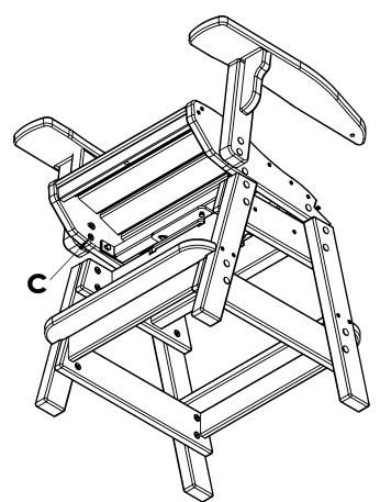
**10.** Attach the two arm assemblies from steps 6-9 to the seat base using hardware c
