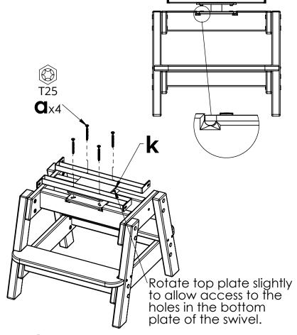
**4.** Attach Hardware k to the previous assembly using Hardware a
