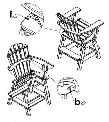
**11.** Attach Back Assembly L to the seat base using hardware f. Attach the Back Assembly center support to each arm using hardware b
