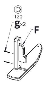
**8.** Place Part F into the pre cut slot and attach with Hardware g
