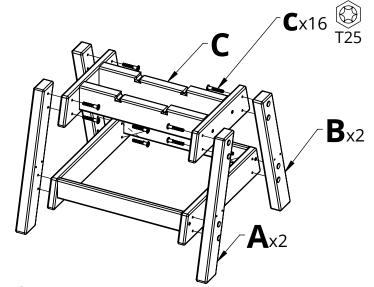
**2.** Connect Parts A & B to Part C & previous assembly using Hardware c
