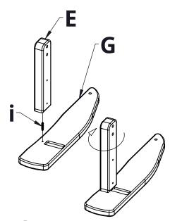
**6.** Attach Part E to Part G using Hardware i
