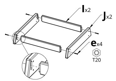
**1.** Connect Parts I & J together using Hardware e
