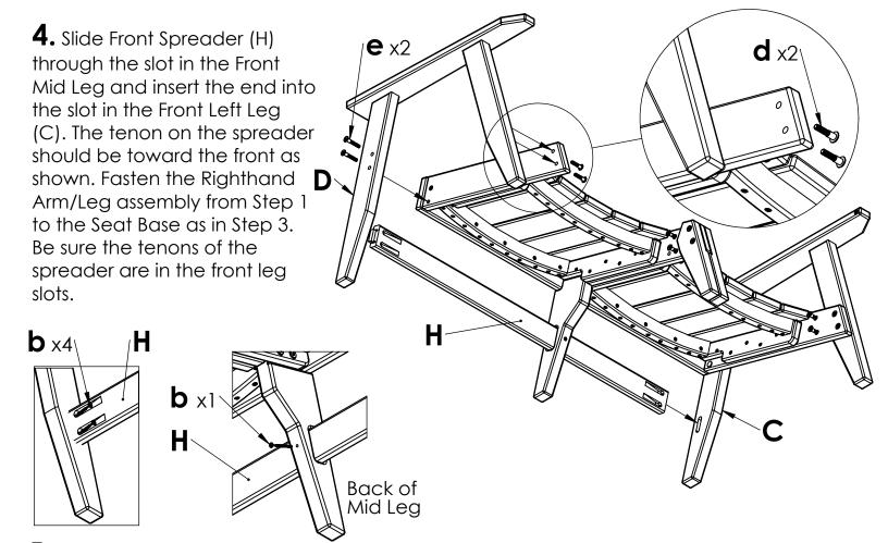
**5.** Turn the assembly from Step 4 onto its front side so the Spreader and Mid Leg holes are face up. Fasten the Spreader (H) to both Front Legs (C & D) using (2) of hardware (b) at the end of each spreader. Use the 6" bit (f) for these screws. Hold the Mid Leg square to the seat front. Fasten it to the Spreader (H) using (1) of hardware (b) - see back of Mid Leg above.
