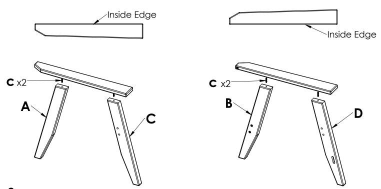
2. Start an end of a double screw (c) in the hole in the top of each leg. Thread the opposite end of the double screw into the corresponding arm, turning the legs clockwise to tighten, until the top of the leg is tight and flush with the bottom of the arm. The slots/threaded inserts in the legs should face toward the inside edge of its corresponding arm.
