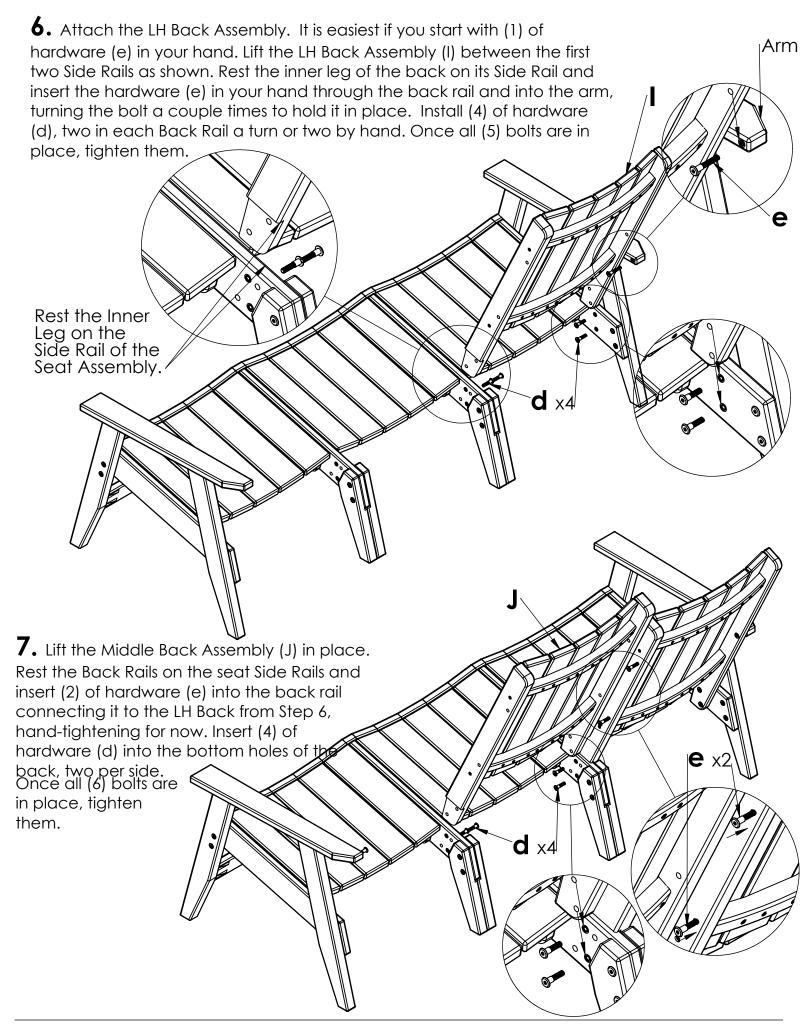
through the Back Rail and into the Arm. Hand-tighten the bolt. Insert (2) hardware (e) through the back rail of the Middle Back Assembly and into the RH Back Assembly and hand-tighten. Insert the remaining (4) hardware (d) into the two holes at the bottom of each Back Rail. Once all (7) bolts are in place, tighten them. Arm e C e
