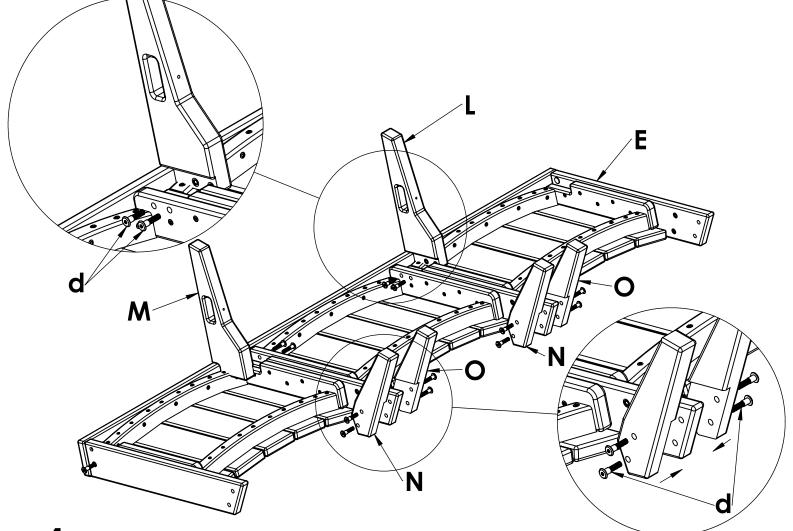
**1.** Turn Seat Assembly (E) upside down on a non-marring surface. Attach Front Mid Legs (L) and (M) using (2) of hardware (d) in each leg - this will require the T25 L-Key due to the limited space. Attach the Mid Back Legs (N) and (O) using (2) of hardware (d) as well.
