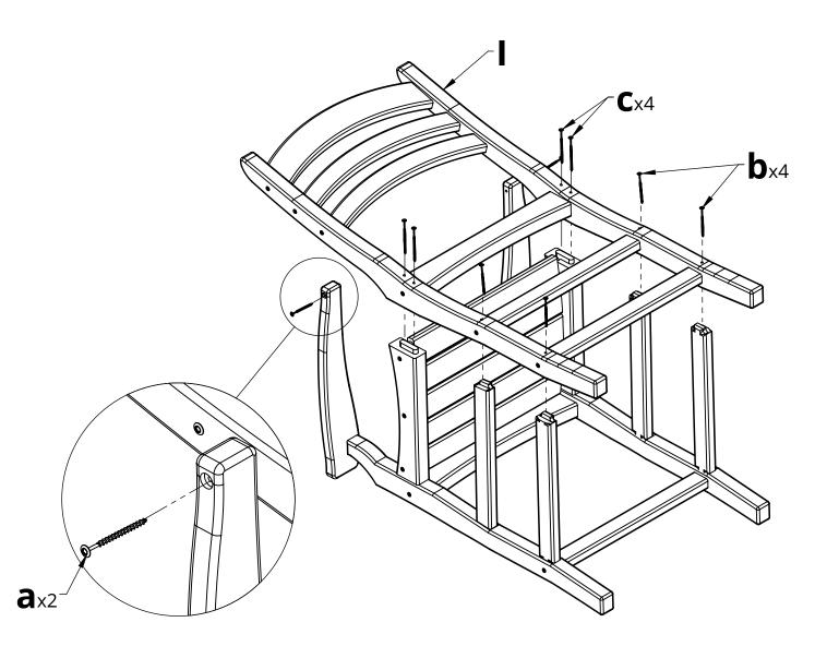
${f 5.}$  Turn the assembly over & attach Part I as shown
