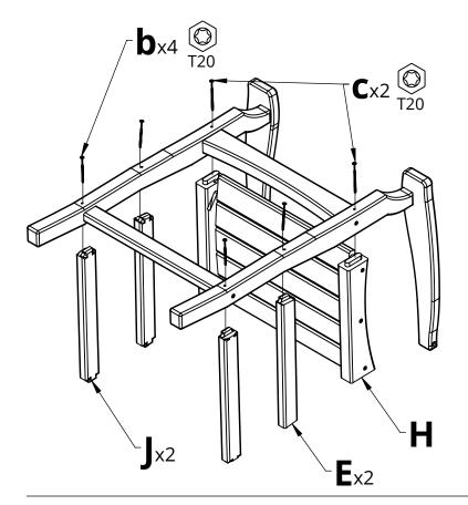
**4.** Insert Parts H, E, & J into the assembly as shown and connect them using the hardware shown
