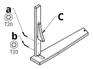
**2.** Connect Part C to the assembly using the hardware shown
