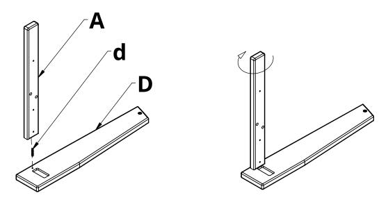
**1.** Attach Part A to Part D by inserting Hardware d into the pre-drilled holes and rotating Part A clockwise, stopping when the assembly is tight
