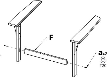
**4.** Attach Part F to the previous assemblies using Hardware a
