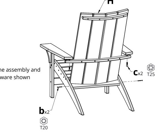
**6.** Slide Part H into the assembly and attach it with the hardware shown
