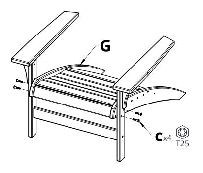
**5.** Place Part G between the previous assemblies and connect it with Hardware c
